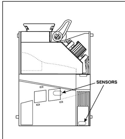
returns the plunger to its de-energized state, which returns the solenoid lever and payout slide, dispensing a coin. Your coin-op regulates the payout rate to ensure proper coin payout reliability.
